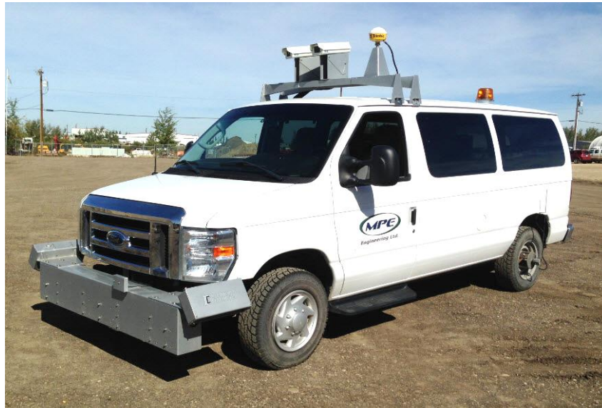
Figure 4.1: MPE Engineering Ltd. Data Collection Vehicle (Class I Profiler)
