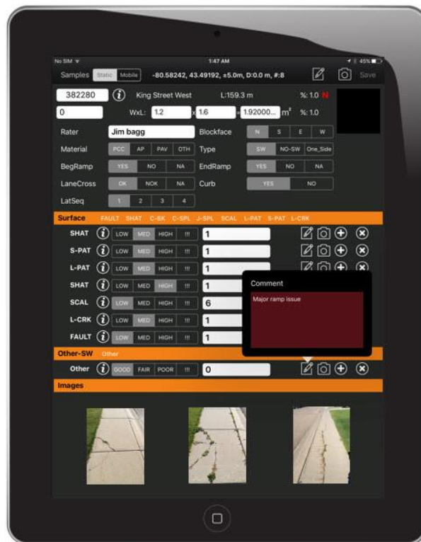
Figure 5.2: MPE rRate Data Collection Tablet (RUBIX)
